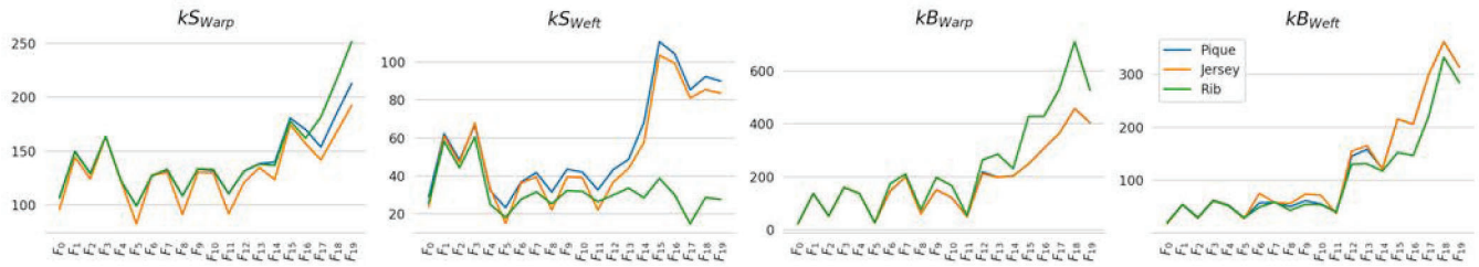
Figure 9: Effect of changing the family of randomly sampled dataset knit fabrics (sorted by density on the horizontal axis) on the output mechanical parameters. The Rib samples tend to decrease resistance to stretch in the weft direction while increase bending resistance in the warp direction w.r.t. the other families, most notably in the denser samples. Pique samples, on the other hand, show slightly higher stretch resistance w.r.t. their Jersey counterparts.
